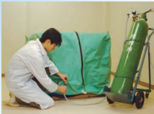
炭酸ガス燻蒸作業風景 Carbon dioxide fumigation system
