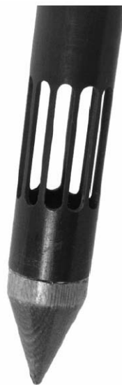
Figure 2. Detail of the intake design used on all of the piezometers. The intake is 7 cm in length
